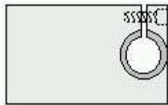
4-40x3/8 socket head cap screw. Use 3/32 Allen wrench.
