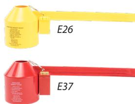
Seedburo hand testers give fast, accurate bulk density readings. Equipped with a sliding beveled poise and a heavy gauge cast anodized aluminum cup. Built to withstand rough use with constant accuracy. Cups should be filled using one of the filling devices shown below. Each unit includes a No. 65 Strike-Off Stick. Net wt: 3 lbs, Ship wt: 4 lbs, Ship dims: 6" (L) x 6" (W) x 15" (H).
