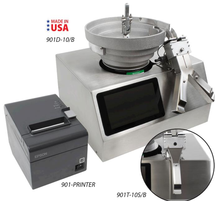
the feeder will stop. Another Batch may be counted by changing the bag or putting a bag on the other chute at this time and pressing START again.
