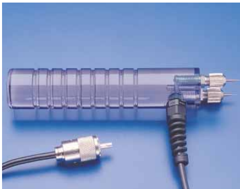
22-E Two pins, 1/2" penetration. Use on plaster, masonry and wood. Will also take #496, insulated pins; 1 1/16" penetration.
