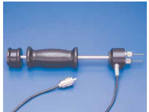
26-ES Two pins, 1 1/16" penetration. Use to measure moisture content in wood at different levels of penetration. Ideal for shell and core tests to detect moisture gradients and to test lumber with wet surfaces.
