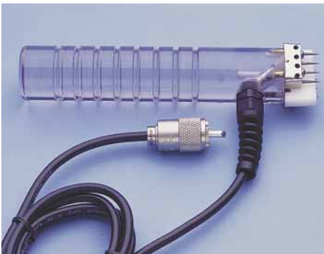
15-E Eight pins, 1/8" penetration. Use on veneer, cardboard, leather, paper.
