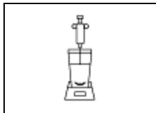
2. Remove an aliquot of homogenate with Syringe Pipet, or Weigh into Bottle.
