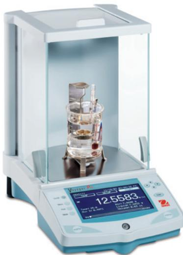
An accessory density determination kit is designed to be used with OHAUS Voyager *Pro* balances. A built-in reference density table for water at temperatures between 10°C and 30°C is included in the balance software. When making density measurements, the material should weigh at least 10.0 mg on an analytical balance and 100 mg on a precision balance.
